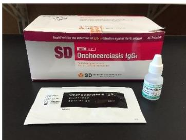
Ensure test cassettes and chase buffer are at ambient temperature before performing tests.
