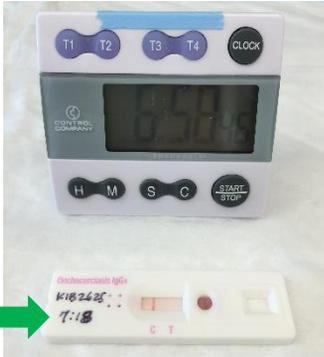
Record reading time directly on the cassette to ensure results are read at the appropriate time
