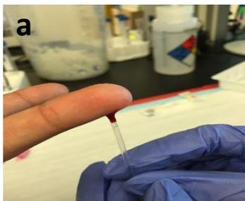
When testing with blood directly from a finger stick use the 10µl micropipette provided (a); fill micropipette to the blue line.
